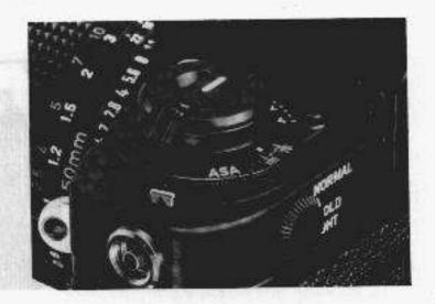
Turn the setting dial, while pressing the lock release button, until the desired film speed aligns with the index. The dial cannot be turned lower than ISO 6 or higher than ISO 6400. The table on the next page shows the ISO film speeds which can be set on the Canon F-1. Figures in parentheses are intermediate speeds which are indicated by dots on the ISO dial.
