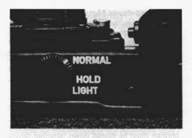
HOLD: The meter turns on the moment you press the shutter button half-way and stays on for 16 seconds even if you remove your finger from the shutter button. It automatically turns off after the specified time, thus conserving battery power. This mode is particularly suited for manual exposure and any situation in which you need more time to meter.
