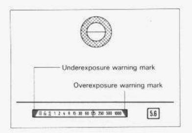
the meter needle indicates a shutter speed of 1/30 sec. or slower. In this case, choose a larger aperture until the shutter speed indicated is 1/60 sec. or faster. If you have set the maximum aperture and the shutter speed is still slower than 1/60 sec., attach the camera to a tripod, use a flash or add artificial light.
