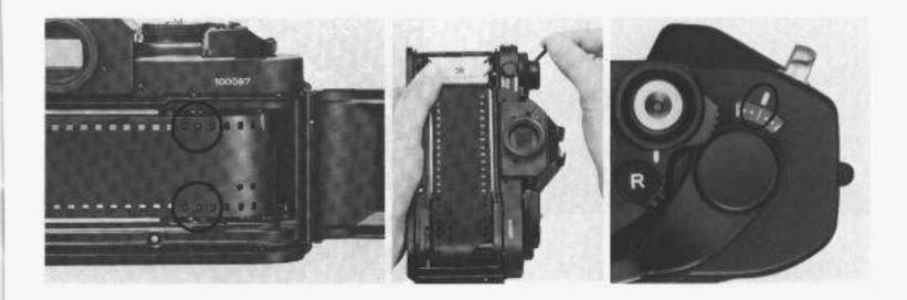
Pull the film leader across the camera and insert the tip into any slot of the take-up spool.
