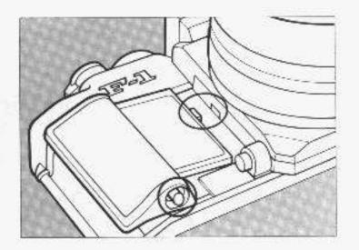
To ensure proper contact, wipe the battery terminals with a clean, dry cloth before loading. Load a new battery so that its terminals are in the directions indicated by the diagram inside the battery chamber. Insert the negative end first, then push down and insert the positive end. The camera will not function if the battery is loaded incorrectly.
