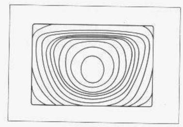
With the Canon F-1, a special optical element in each focusing screen determines the metering sensitivity area. Thus the metering area can be changed, according to the subject you are shooting and the lens in use, simply by replacing the focusing screen.
