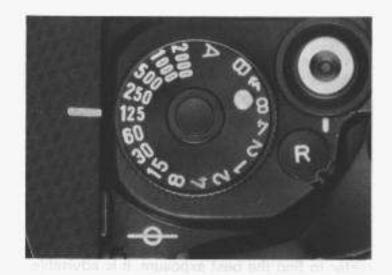
The Canon F-1's hybrid shutter is electronically as well as mechanically controlled. Shutter speeds from 1/2000 to 1/125 sec., "#" (1/90 sec.) and "B" (bulb) are mechanically governed, while 1/60 to 8 secs. are electronically controlled. With the AE Finder FN attached and the shutter dial on "A" shutter speeds from 1/1000 to 8 secs. are electronically controlled.
